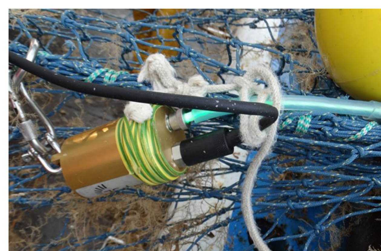
The Photosynergy Ltd light pod with side emitting fibre optic cable
