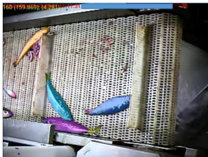
Figure 2. Convolutional neural network identification of fish passing along a discard belt, with running count (top left) of the number recorded going overboard. A demonstration of the system can be viewed at:
