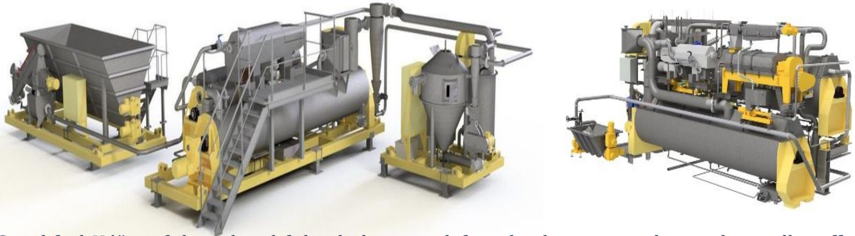
Simplified Héðinn fishmeal and fish oil plants, on left on land version and on right smaller off-shore version.
